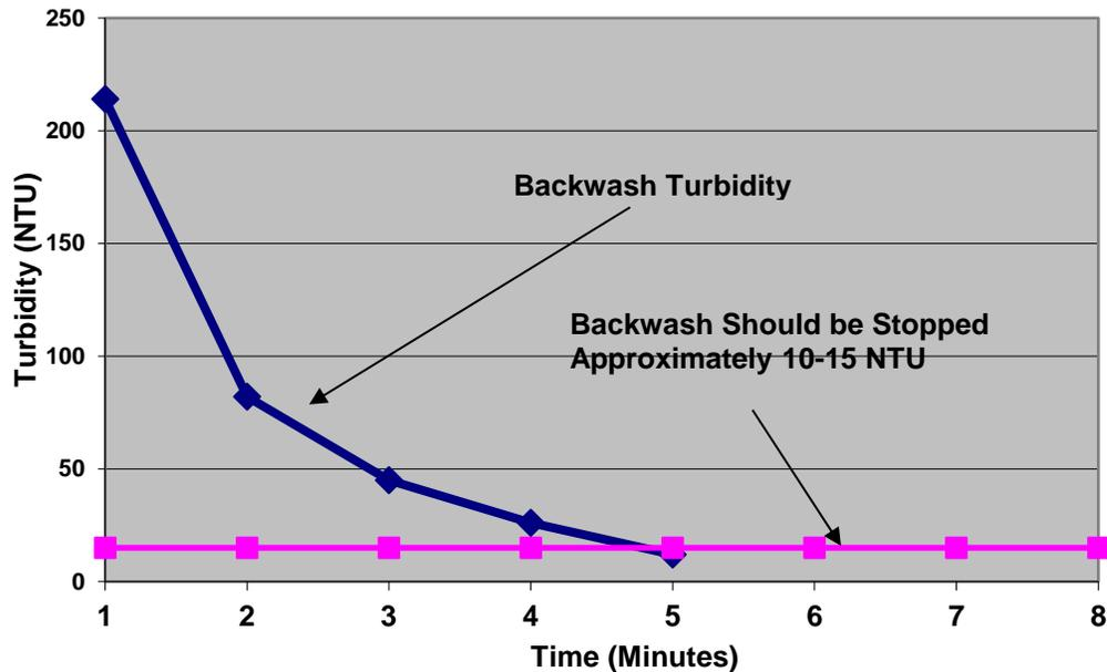
Figure 7 – Spent Filter Backwash Water Turbidity Profile
