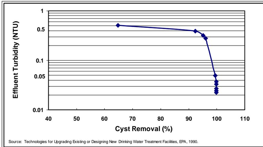
**Figure 1 – Percent Cyst Removal vs. Filtered Water Turbidity**
