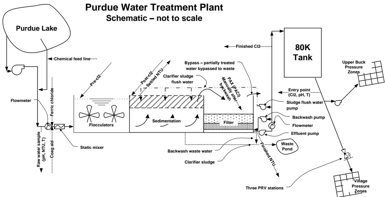
Figure 3 – Schematic of PWTP
